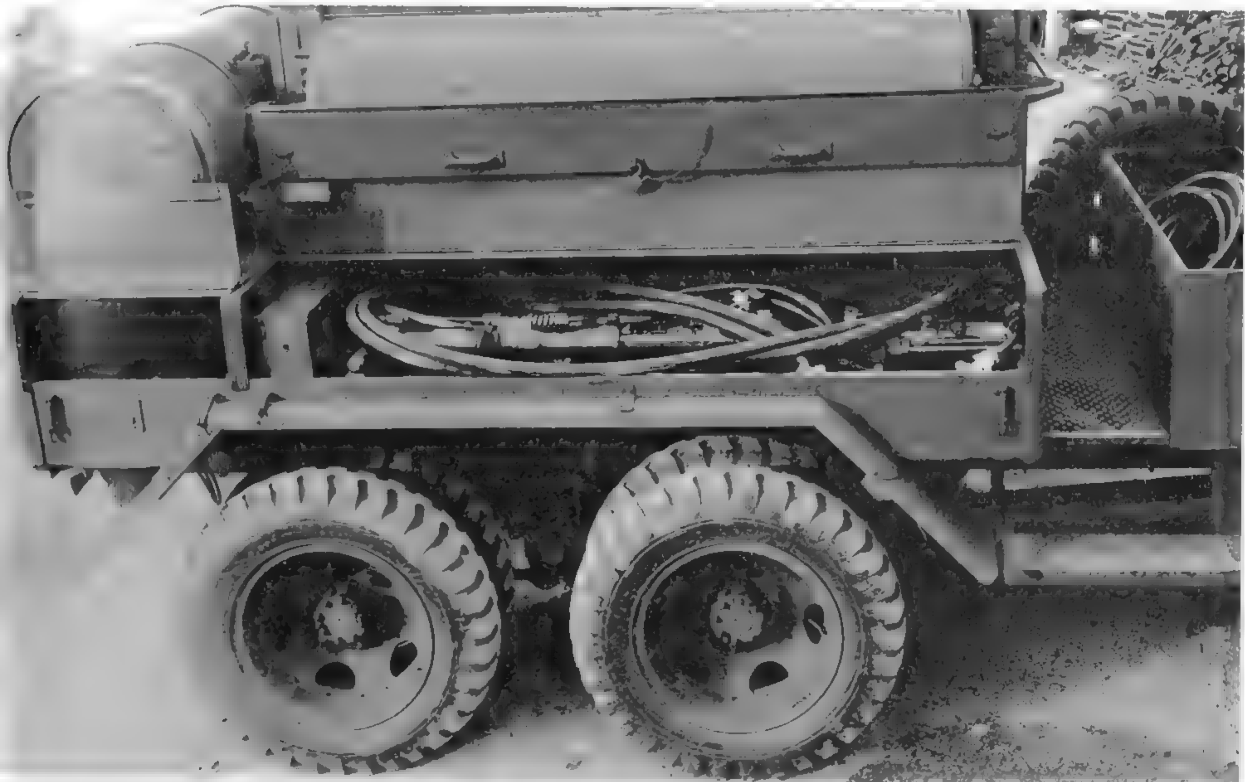
The tool compartments alongside the Le Roi 105G compressor held a variety of pneumatic construction tools. The compressor had a capacity of 105 cu. ft. per minute, and was powered by its own four-cylinder engine. (Photo courtesy of U. S. Army Engineer School History Office)
